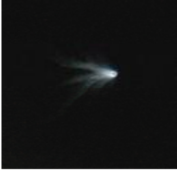
Figure 2. DC corona discharges
